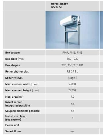
Security level 2: Roller shutter system with integrated anti-push-up device up to 750 N. Certified according to guideline TR 111 of the Bundesverband Rollladen und Sonnenschutz (BVRS)
