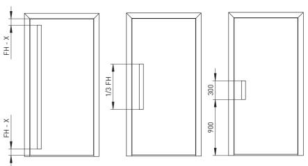
Depending on whether the casement design is flush or protruding, the corresponding bar handle is chosen. They differ with respect to their installation depth:
