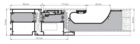
Bar handle depth for flush casement: 37.5 mm
